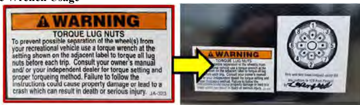
Lug nut torque pattern and warning label
