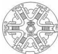
7-way trailer plug car end, rear view
